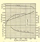
Fig. 281.—Typical internal-combustion-engine performance graphs. (This shows the performance of a 225-h.p. Westinghouse vertical gas engine.)
